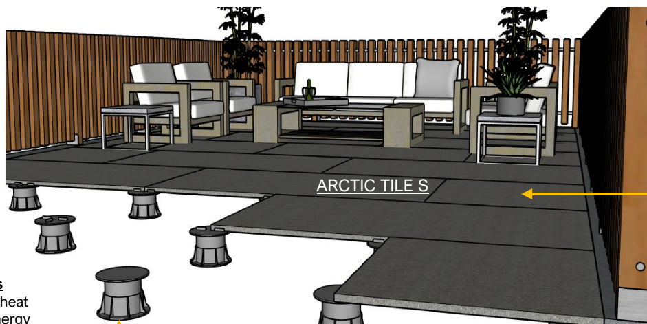
Pedestal Installation Method (Bison Pedestal System can be supplied)
